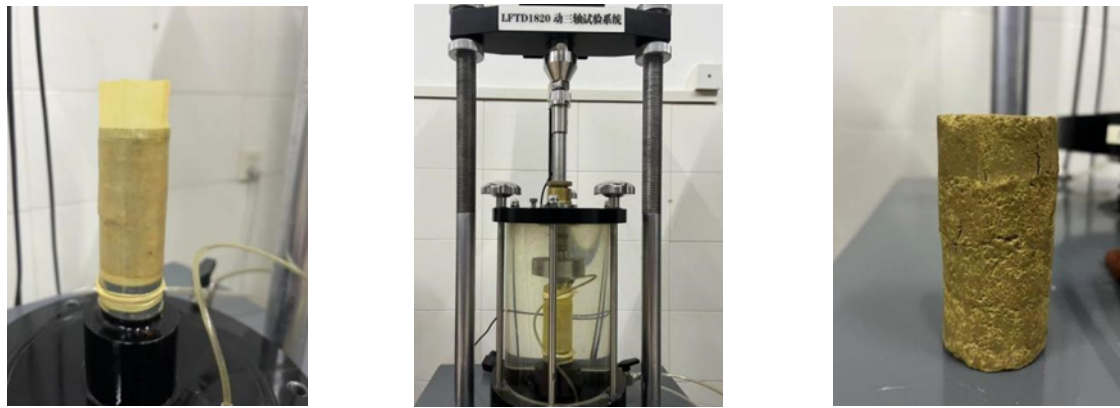
(d) Specimen installation stage (e) Loading stage (f) Specimen failure
