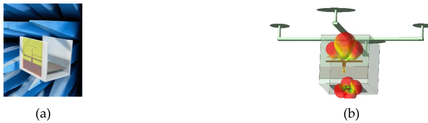
Figure 11: Multimode Pattern Reconfigurable Conformal Antenna (a) Antenna prototype; (b) Radiation beam Pattern.
