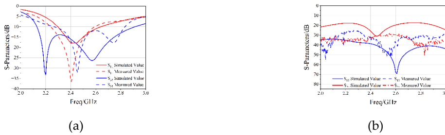
Figure 12: S-parameters of the Simulated and Tested Multi-mode Pattern Reconfigurable Conformal Antenna: (a) Reflection Coefficient; (b) Port Isolation.
