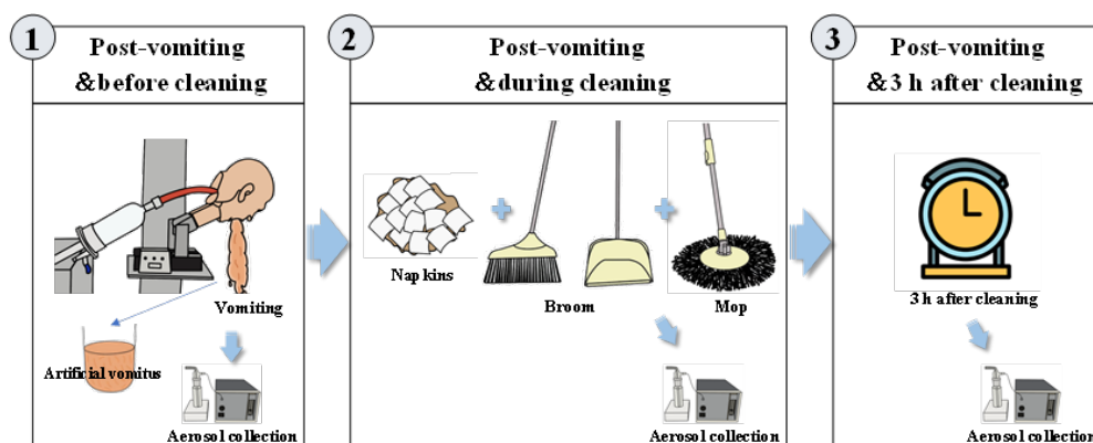
Figure 1: Schematic Diagram of the Air Sample Collection Stage.
